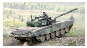
smoothbore gun, which can also fire guided missiles through the tube in the more recent variants. The 125mm gun also uses an automatic loader system, which allowed the Russians to keep the crew to three men. Overall, the T-72 shows the typical even balance between firepower, mobility and protection followed by the Soviet and then the
