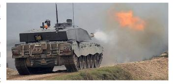
temporarily creates a thick cloud of dust and flames which obscures the sights of the tank gunner for a few seconds, impeding accurate rapid fire. Some tank guns, mostly Russian 125mm models, can fire anti-tank guided missiles through the gun tube.
